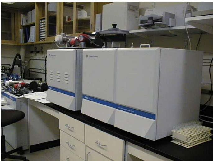
**Figure 4: Elemental analyzer and stable isotope mass spectrometer utilized in this study.**
