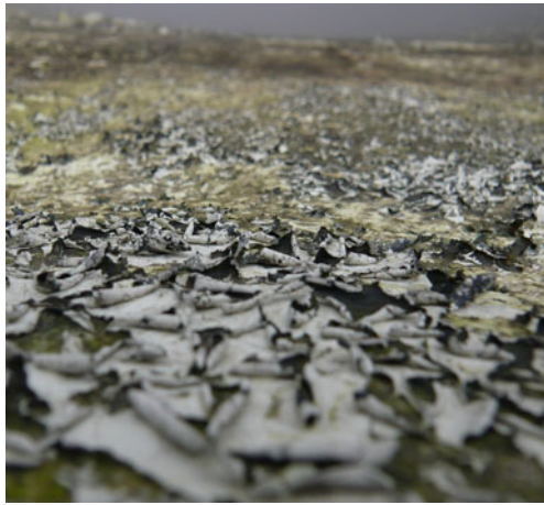
Fig. 3 Drying biofilm with pieces of protective paint on its bottom side
