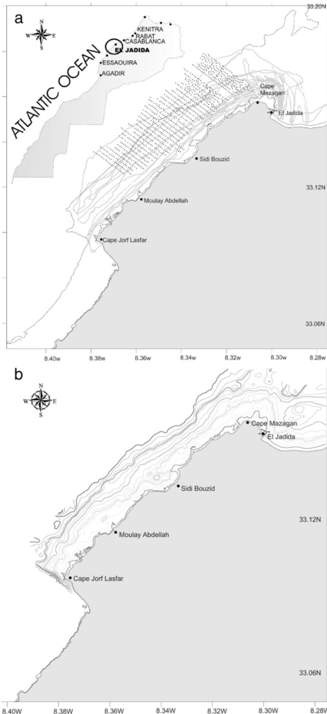
**Fig. 1a.** Data used to construct bathymetric charts. Lines indicate the route of the boat. Dots represent the sampling points for bathymetric modelling.
