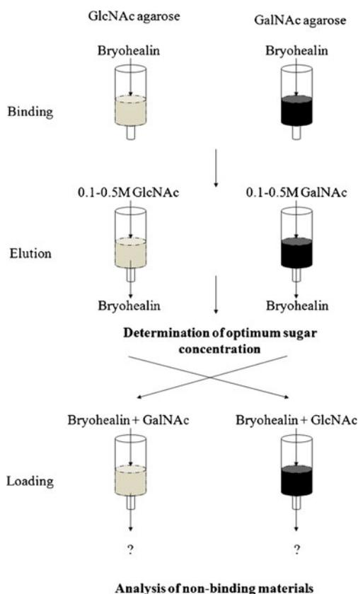
**Fig. 1** Scheme of chromatographic methods for the determination of binding sites
