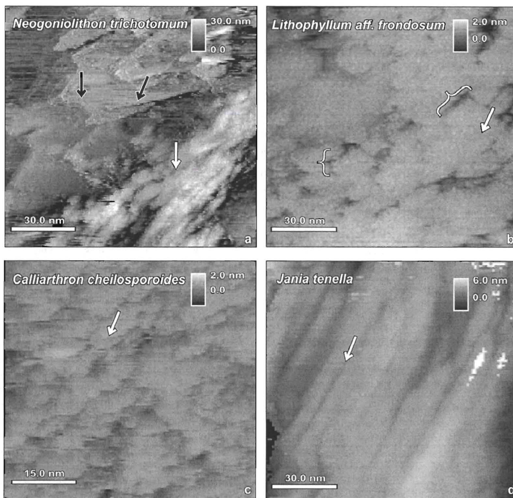
Figure 3. Scanning tunneling microscopy of ground samples of four coralline red algae deposited onto pyrolytic graphite. In Neogoniolithon trichotomum (a) the crystallites do not look structurally homogeneous and are not very regular in shape although clearly needle-like structures; the higher brightness compared with the other images can be due to the presence of non-conductive organic material. The Lithophyllum aff. frondosum (b) image shows plate-like crystallites (brackets) that are very smooth in surface and relatively homogeneous in structure. In Calliarthron cheilosporoides (c) the crystallites have less symmetry and it is possible to observe grooves that can be crystalline planes. In Jania tenella (d) the crystals are clearly bigger than those observed in the other images, and are very homogeneous in surface and in size.
