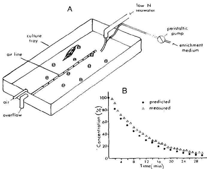
Fig. 3. Detail of culture tray in Fig. 2 (A) and graph (B) showing the predicted and experimentally determined rates of dilution of dye in the culture tray: predicted rate from  $C_t = C_0 e^{-rt}$ , where  $C_t$  = final dye concentration,  $C_0$  = initial dye concentration,  $t$  = time and  $r$  = dilution rate.
