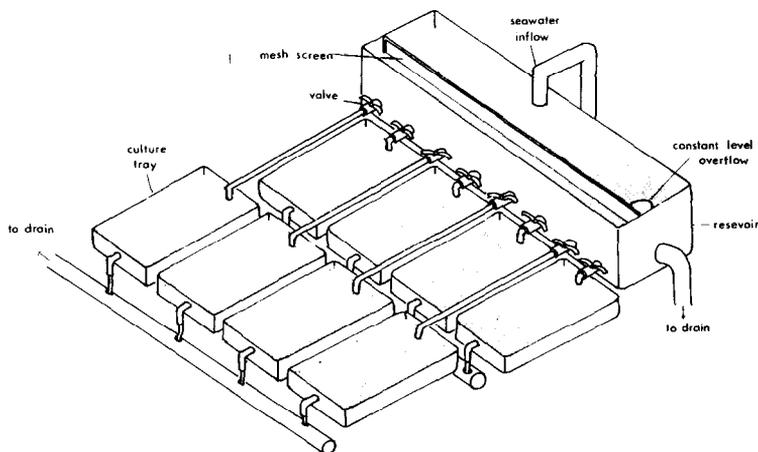
Fig. 2. Layout for rapid flushing outdoor cultivation experiments.
